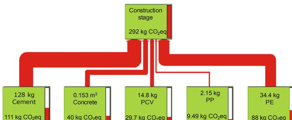
Fig. 3. Determinants of GHG emission for individual wastewater treatment plants, stage of construction, kg CO<sub>2</sub> eq/FU
