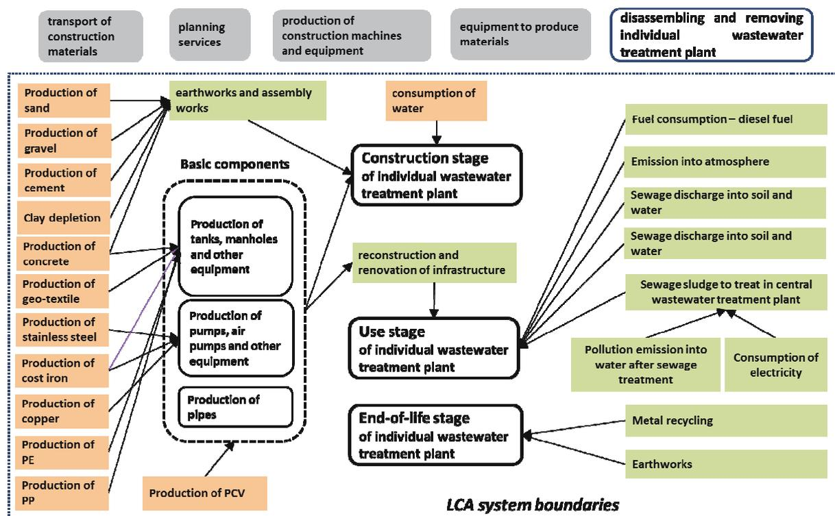
Fig. 2. System boundaries of life cycle assessment of individual wastewater treatment plant
