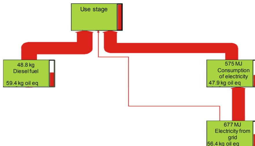
**Fig. 5.** Determinants of fossil fuel depletion for IWWTPs, use stage, kg oil eq/FU
