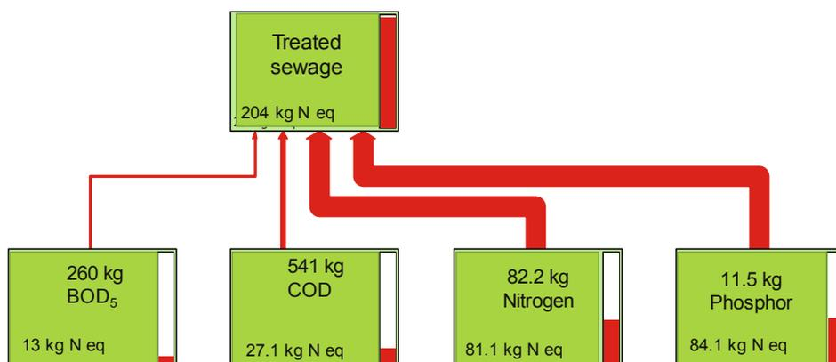
Fig. 6. Main sources of eutrophication resulting from using IWWTPs
