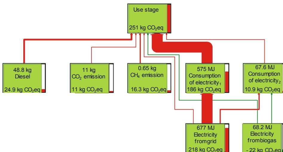
Fig. 4. Determinants of GHG emission for individual wastewater treatment plants, use stage, kg CO<sub>2</sub> eq/FU
