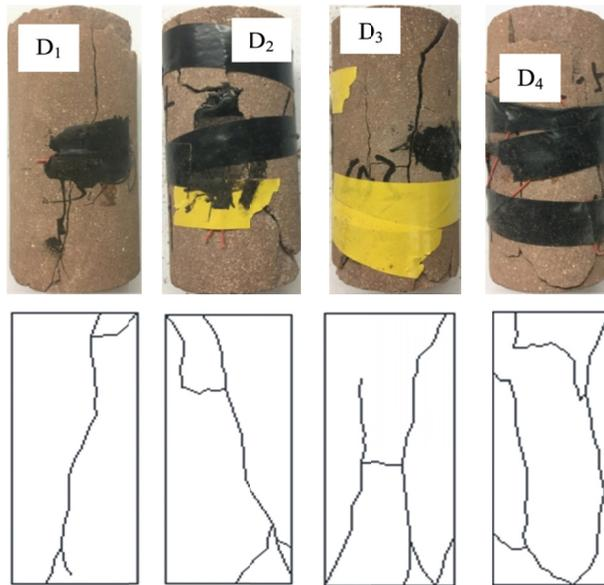
Fig. 7. Typical failure morphologies of the rock specimens
