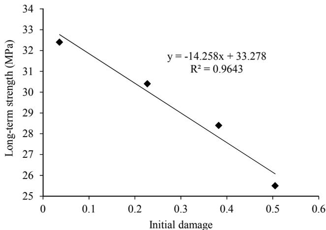
Fig. 16. Relation between long-term strength and initial damage
