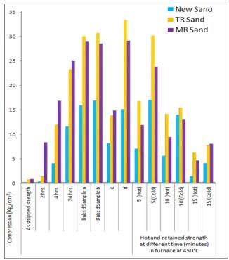
Fig. 11. Recipe: 0.8:50 Medium Fast Catalyst RT-20°C, RH-47%
