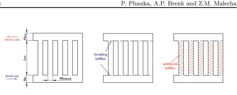
Figure 2: Schematic of characteristic features used in 2D geometry of PHE to model its 3D original: a) basic dimensions of 2D PHE; b) placement of throttling baffles; c) additional baffles modeling complexity of the flow of the 3D PHE.
