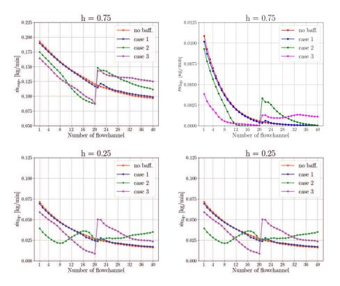
Figure 11: Distribution of R410A vapor (left) an liquid (right) mass flows across the PHE flow channels for different baffle modifications (including baseline). Stabilized solution for simulated time of 10 s. Section taken from the 75% and 25% of the PHE height.
