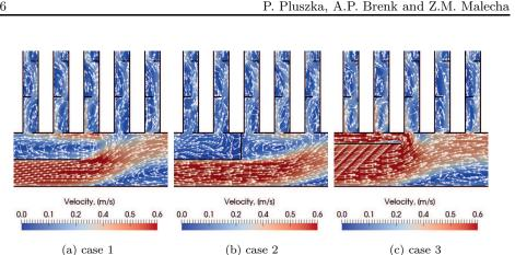
Figure 12: Local flow pattern near baffle's end.
