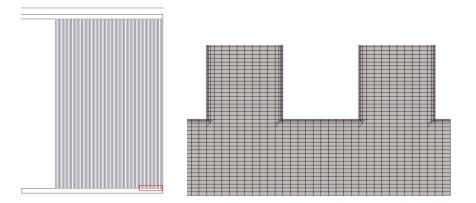
Figure 6: Domain (left) and mesh close-up (right) for the geometry of 40 flow channels.
