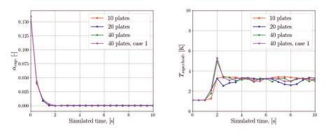
Figure 7: Comparison of investigated PHE cases in terms of the volumetric liquid fraction and superheated temperature at the PHE outlet.
