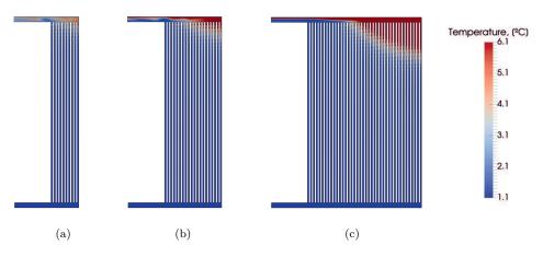
Figure 10: Temperature distribution in the exchanger for: a) 10, b) 20, c) 40 flow channels. Stabilized solution for simulated time of 10 s.
