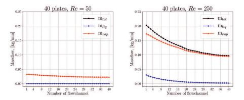
Figure 9: Comparison of mass flow distribution for the 40 plates PHE cases between the systems characterized by Reynolds number Re = 50 (left) and Re = 250(right). Section taken from the half-height of exchanger.
