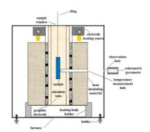
Fig. 3. A schematic diagram of the moderate-temperature chamber.
