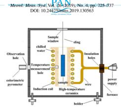
Fig. 2. A schematic diagram of the high-temperature chamber.
