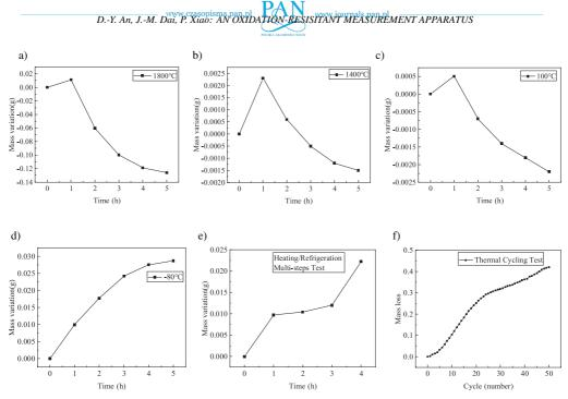
Fig. 9. Relationship between mass variation of a specimen and test time or number of thermal cycling tests: a) hightemperature test; b) moderate-temperature test; c) normal-temperature test; d) low-temperature test; e) multi-step oxidation test; f) thermal cycling test.
