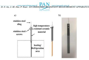
Fig. 6. A schematic of the high-temperature oxidation-resistant chuck. a) Structure; b) actual object.
