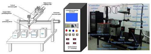
Fig. 1. An overview of test apparatus.
