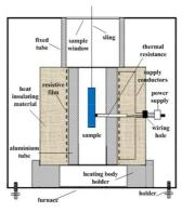
Fig. 4. A schematic diagram of the normal-temperature chamber.
