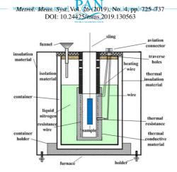
Fig. 5. A schematic diagram of the low-temperature chamber.
