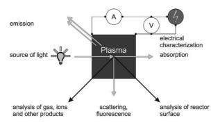
Fig. 3. Methods of micro-plasma characterization (based on [11]).
