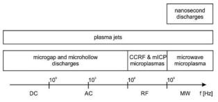
Fig. 2. Classification of micro-plasma sources (based on [11]).
