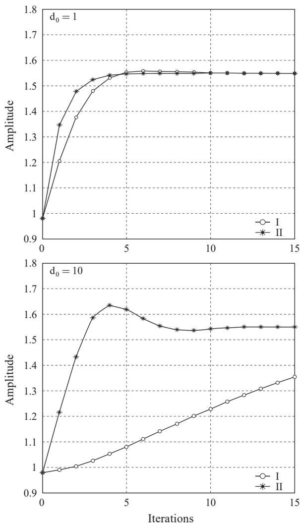
Fig. 3 Amplitude of current wave-forms for successive iterations at  $\Omega = 1,0, d_0 = 1,0$  and  $d_0 = 10,0$ ; curve I – Algorithm 1, curve II – Algorithm 2
