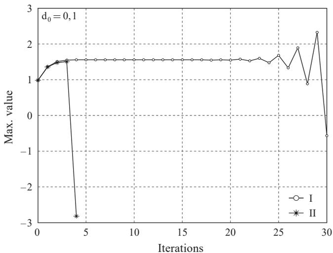
Fig. 2a Amplitude of current waveform for successive iterations at  $\Omega = 1,0, d_0 = 0,1$ ; curve I – Algorithm 1, curve II – Algorithm 2
