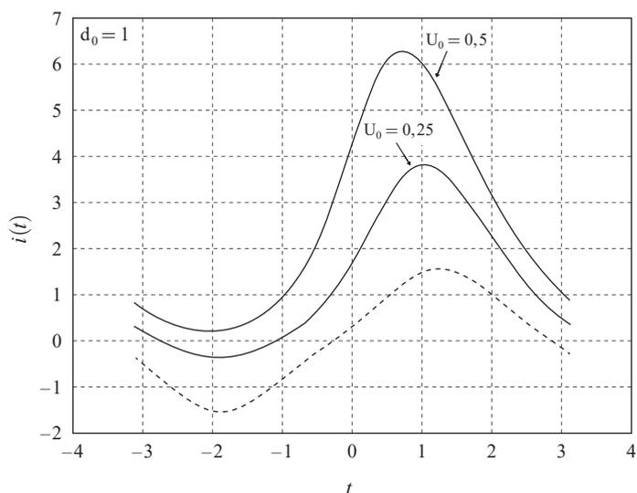
Fig. 6 Final current wave-forms at  $U_m = 1,0$  [V],  $U_0 = 0,25$  [V] and  $U_0 = 0,5$  [V]
