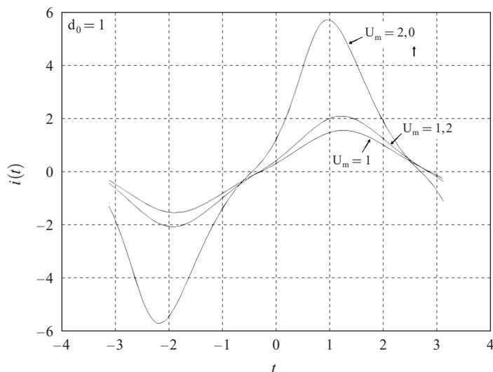
Fig. 5 Final current wave-forms for  $U_0 = 0,0$  [V],  $U_m = 1,0$  [V],  $U_m = 1,2$  [V] and  $U_m = 2,0$  [V]
