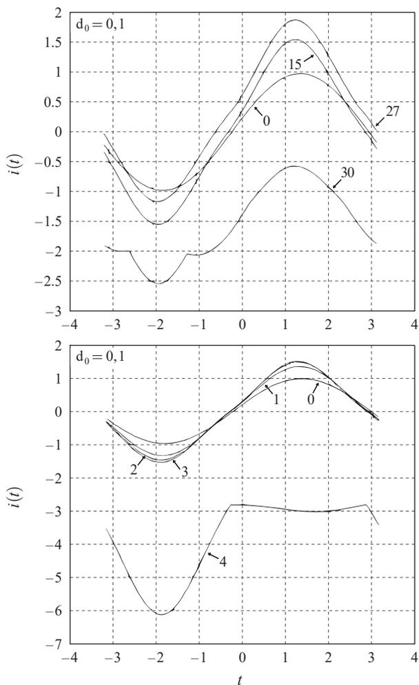
Fig. 2b Current wave-forms for selected iterations at  $\Omega = 1,0, d_0 = 0,1$ ; left – Algorithm 1, right – Algorithm 2
