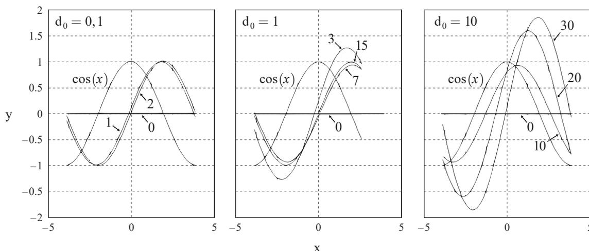
Fig. 1a. Wave-forms for selected iterations at  $\Omega = 1,0$ ,  $d_0 = 0,1$ ,  $d_0 = 1,0$  and  $d_0 = 10,0$
