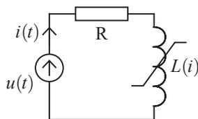
Fig. 2 Elementary circuit with nonlinear coil
