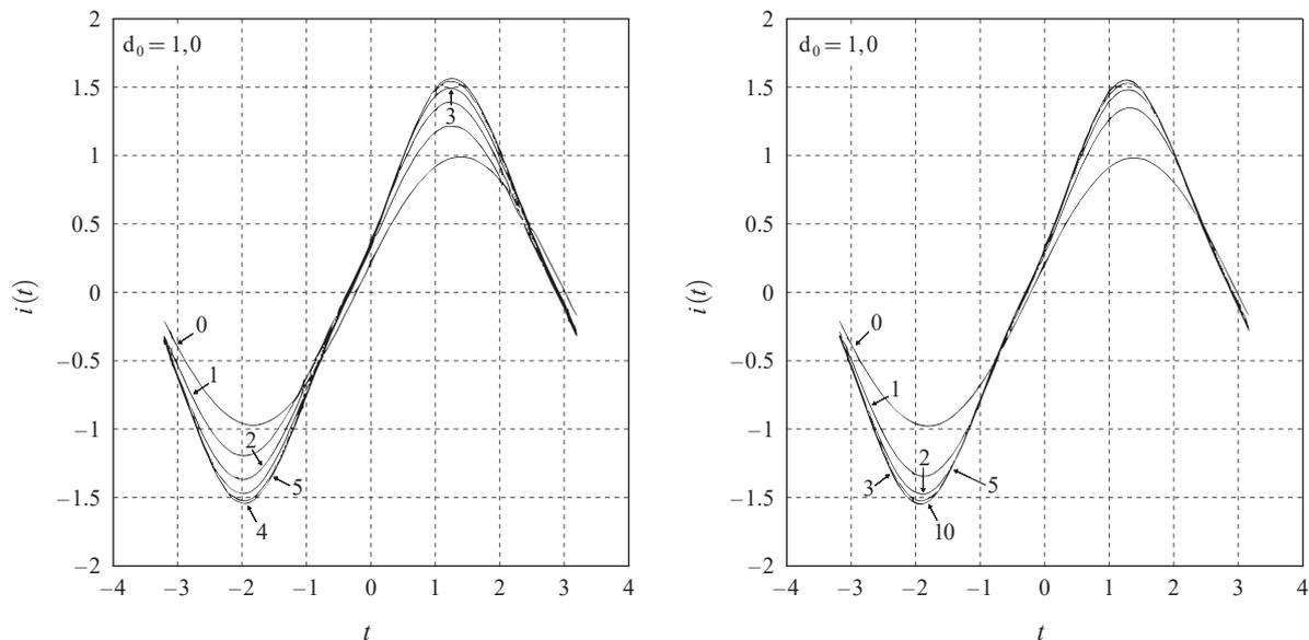
Fig. 4 Current wave-forms for successive iterations at  $\Omega = 1,0$ ,  $d_0 = 1,0$  curve I – Algorithm 1, curve II – Algorithm 2
