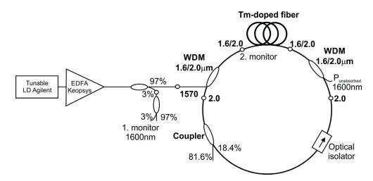
Fig. 1. Ring fiber laser setup used for characterization
