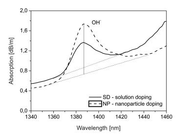
Fig. 4. Attenuation of fibers fabricated by both the conventional SD method and by the NP method in the spectral region corresponding to OH<sup>-</sup> absorption
