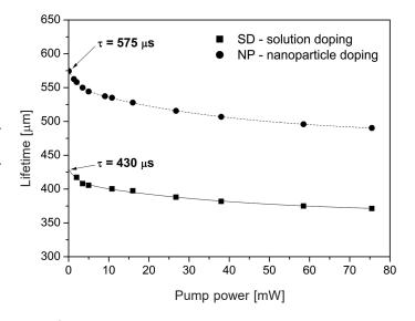
Fig. 5. <sup>3</sup>F<sub>4</sub> lifetime of fibers fabricated by the conventional SD method and the NP method
