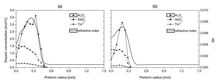
Fig. 2. Refractive-index and concentration profiles of preforms prepared by means of a) the conventional SD method, b) the NP method
