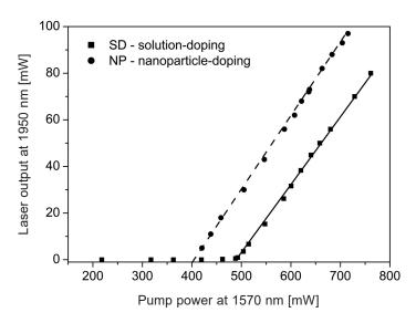
Fig. 6. Ring laser output characteristics measured from fibers fabricated by both the conventional SD method and the NP method
