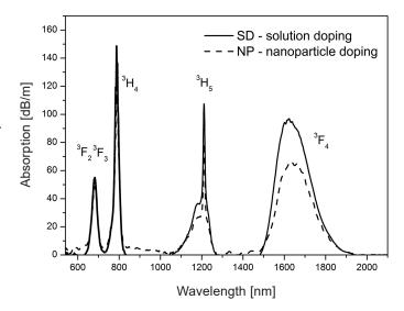
Fig. 3. Spectral attenuation of thulium-doped fibers drawn from preforms fabricated by both the conventional SD method and the NP method
