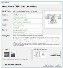
Fig. 4. Main interface of the Open Atlas of Defects
