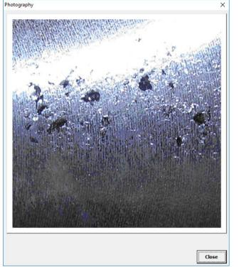
Fig. 5. Example of visualisation of the "shrinkage porosity" defect in the Open Atlas of Defects
