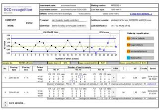
Fig. 7. DCC card – an example of process quality management with three kinds of defects (assortment 530124359)
