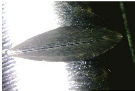
Fig. 6. Close view of the fatigue crack at the tip of the notch on the shaft
