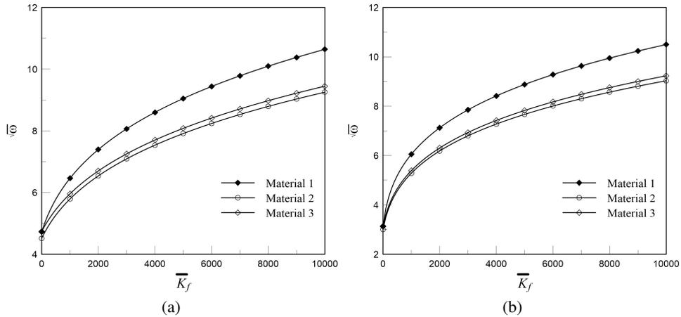
Fig. 3. Effect of different material models on natural frequency of FGM beam (a) clamped-clamped, (b) simply supported-simply supported
