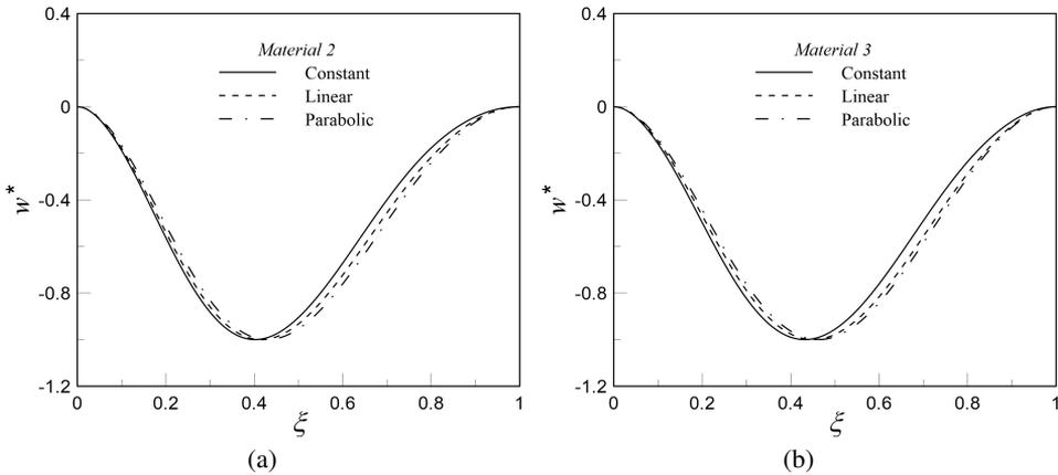
Fig. 6. Effect of variable foundation on the mode shapes of CC FGM beam (a) *Material 2* (b) *Material 3*
