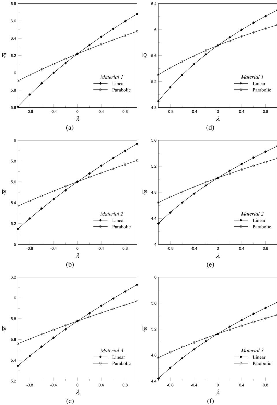
Fig. 5. Effect of foundation stiffness parameter ( $\lambda$ ) on natural frequency of FGM beam (a, b, c) clamped-clamped, (d, e, f) simply supported-simply supported
