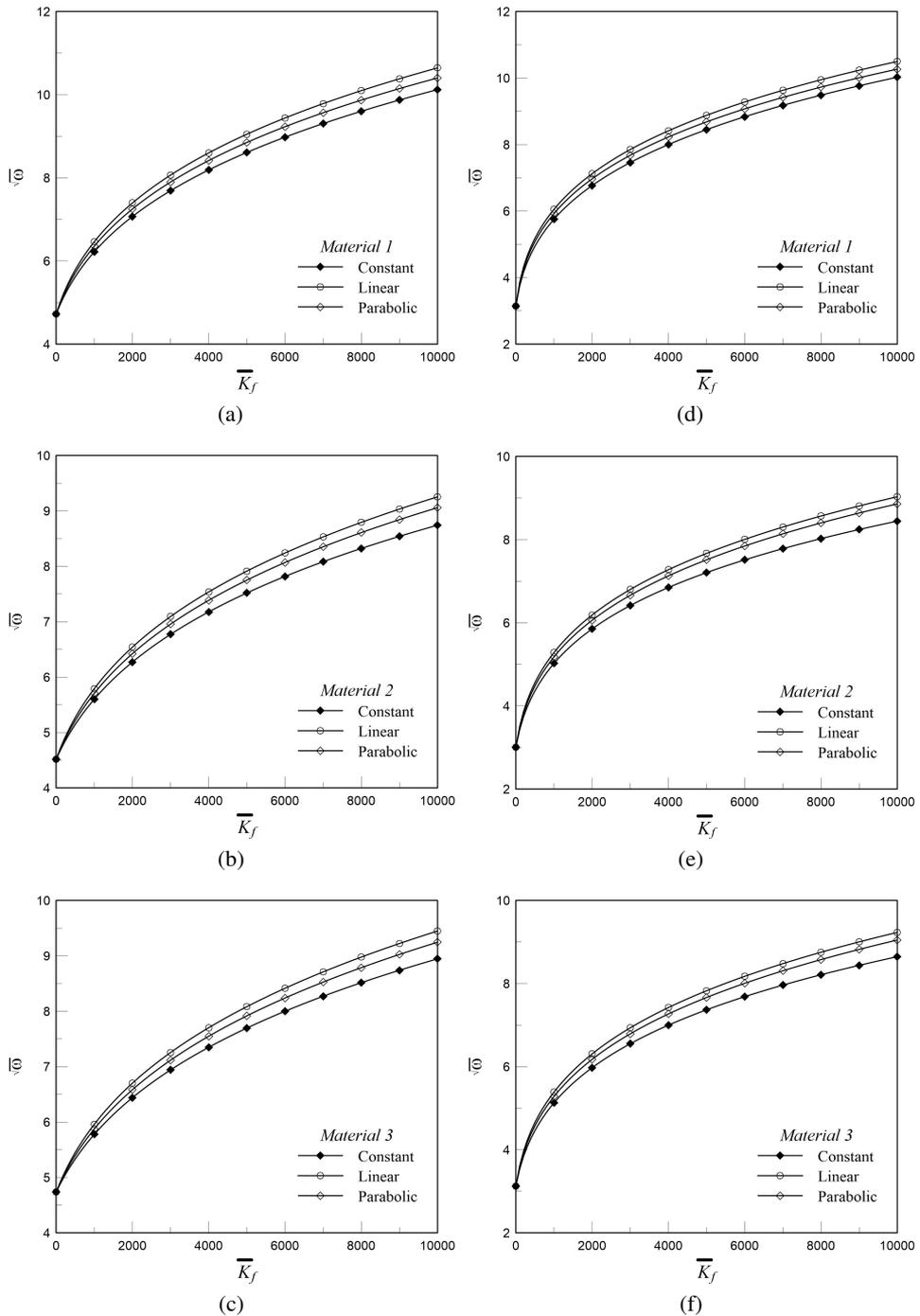
Fig. 2. Effect of foundation stiffness on natural frequency of FGM beam (a, b, c) clamped-clamped, (d, e, f) simply supported-simply supported
