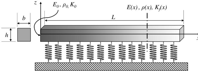
Fig. 1. FGM beam resting on Winkler foundation
