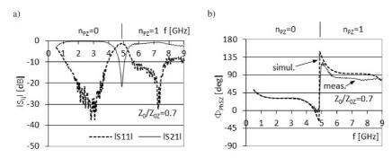
Fig. 13. The measured amplitude characteristics (a), and the differential phase shift  $\Phi_{PhSZ}$  (b), of a microwave phase shifter with a parallel short-circuited stub for  $Z_0/Z_{0Z} = 0.7$  ( $w_{SZ} = 1.36$  mm,  $L_{SZ} = 17$  mm,  $L_{Ref} = 70$  mm).
