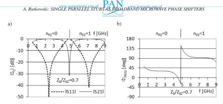
Fig. 7. The amplitude characteristics (a), and the differential phase shift  $\Phi_{PhSZ}$  (b), of a microwave phase shifter with a parallel short-circuited stub for  $Z_0/Z_{0Z} = 0.7$  (results of simulations,  $L_{Ref} = 70$  mm).
