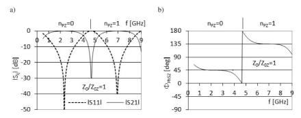
Fig. 6. The amplitude characteristics (a), and the differential phase shift  $\Phi_{PhSZ}$  (b), of a microwave phase shifter with a parallel short-circuited stub for  $Z_0/Z_{0Z} = 1$  (results of simulations,  $L_{Ref} = 74.5$  mm).
