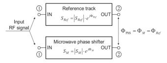
Fig. 1. A symbolic composition of a microwave phase shifter and a reference track to demonstrate *differential phase shift*  $\Phi_{PhS}$ .
