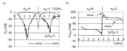
Fig. 12. The measured amplitude characteristics (a), and the differential phase shift  $\Phi_{PhSZ}$  (b), of a microwave phase shifter with a parallel short-circuited stub for  $Z_0/Z_{0Z} = 1$  ( $w_{SZ} = 2.73$  mm,  $L_{SZ} = 17$  mm,  $L_{Ref} = 74.5$  mm).
