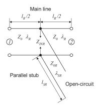
Fig. 2. A microwave phase shifter with a single parallel open-circuited stub.
