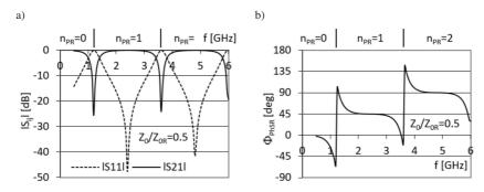
Fig. 4. The amplitude characteristics (a), and the differential phase shift  $\Phi_{PhSR}$  (b), of a microwave phase shifter with a parallel open-circuited stub for  $Z_0/Z_{0R} = 0.5$  (results of simulations,  $L_{Ref} = 74.5$  mm).
