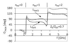
Fig. 14. The measured differential phase shift  $\Phi_{PhSR}$  of a microwave phase shifter with a parallel open-circuited stub for  $Z_0/Z_{0R} = 0.7$  and for two various reference line lengths ( $L_{Ref1} = 80 \text{ mm}$ ,  $L_{Ref2} = 88.7 \text{ mm}$ ).
