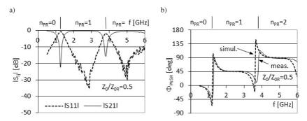
Fig. 10. The measured amplitude characteristics (a), and the differential phase shift  $\Phi_{PhSR}$  (b), of a microwave phase shifter with a parallel open-circuited stub for  $Z_0/Z_{0R} = 0.5$  ( $w_{SR} = 0.68$  mm,  $L_{SR} = 35$  mm,  $L_{Ref} = 74.5$  mm).
