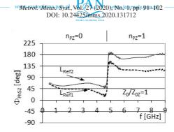
Fig. 15. The measured differential phase shift  $\Phi_{PhSZ}$  of a microwave phase shifter with a parallel short-circuited stub for  $Z_0/Z_{0Z} = 1$  and for two various reference line lengths ( $L_{Ref1} = 74.5$  mm,  $L_{Ref2} = 80.5$  mm).
