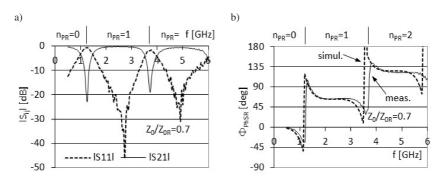
Fig. 11. The measured amplitude characteristics (a), and the differential phase shift  $\Phi_{PhSR}$  (b), of a microwave phase shifter with a parallel open-circuited stub for  $Z_0/Z_{0R} = 0.7$  ( $w_{SR} = 1.37$  mm,  $L_{SR} = 35$  mm,  $L_{Ref} = 80$  mm).
