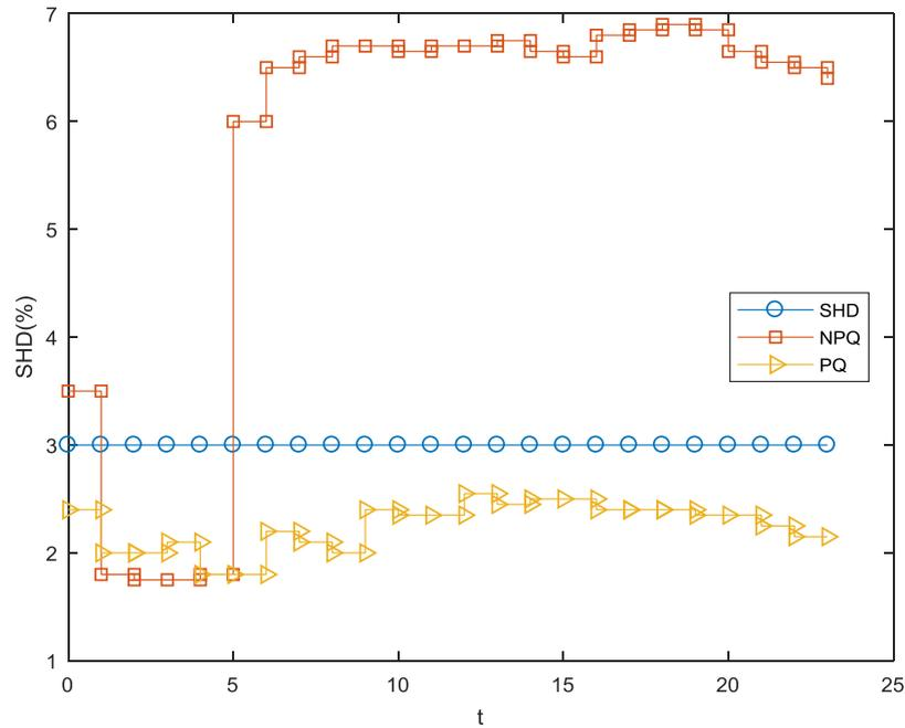
Fig. 5. The maximum single harmonic distortion value per hour under the IEEE 123 node system
