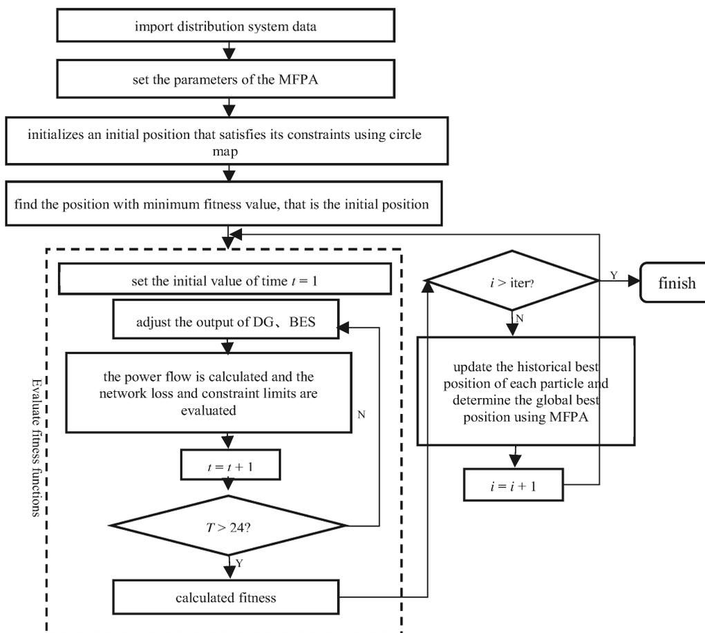
Fig. 2. Flowchart of active distribution network scheduling based on MFPA
