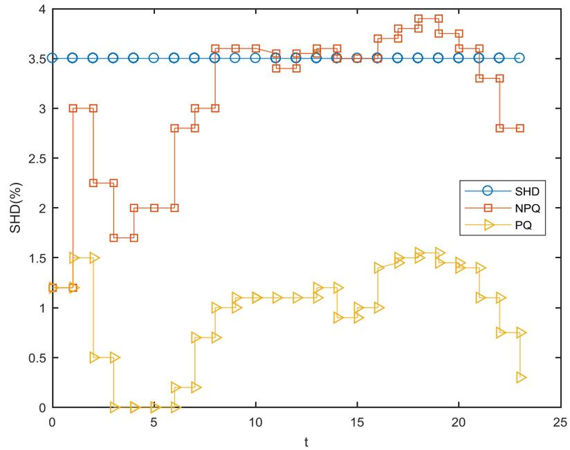
Fig. 3. Maximum single harmonic distortion value per hour in the IEEE 37-node system
