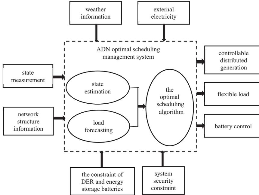
Fig. 1. ADN optimal scheduling management system structure diagram
