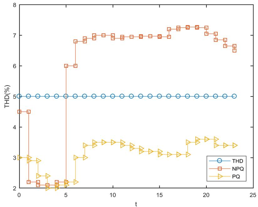
Fig. 4. Total harmonic distortion value of maximum voltage per hour under the IEEE 123 node system
