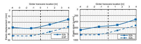
Fig. 7. Transverse distribution of hybrid girder mid-span displacements (left) and strains (right) under the full static load.
