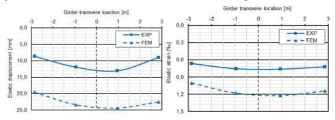
Fig. 5. Transverse distribution of all-composite girder mid-span displacements (left) and strains (right) under the full static load.
