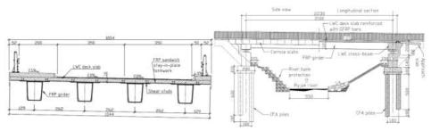
Fig. 2. Cross-section of the hybrid superstructure (left) and side view/longitudinal section (right).
