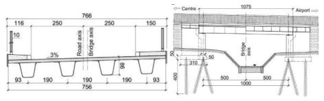
Fig. 1. Cross-section of the all-composite superstructure (left) and side view/longitudinal section (right).
