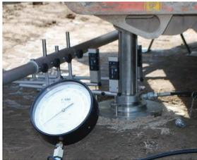
Fig. 10. Static VSS plate measurement
