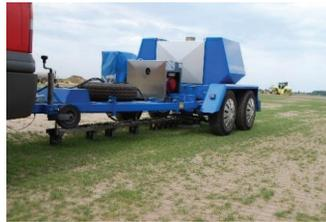
Fig. 11. HWD airfield deflectometer measurement
