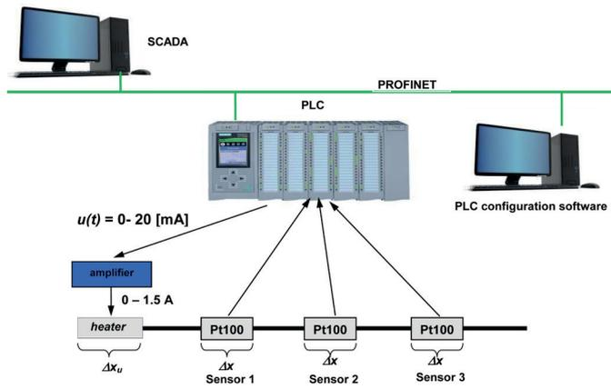
Fig. 2. The construction of the experimental system
