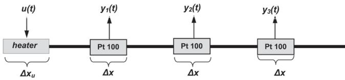
Fig. 1. The simplified scheme of the experimental system
