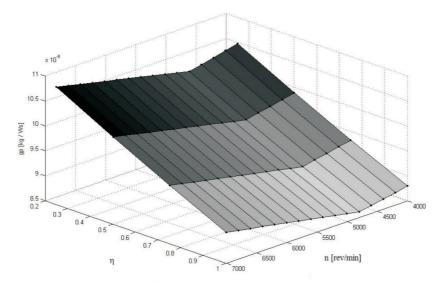
Fig. 3. Specific fuel consumption versus revolutions and power setting
