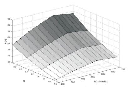
Fig. 2. Power of the engine versus revolutions and power setting
