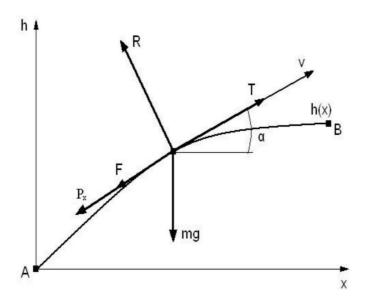
Fig. 1. Particle model of the vehicle
