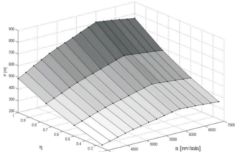
Fig. 2. Power of the engine versus revolutions and power setting
