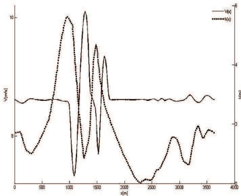
Fig. 6. Optimum velocity versus covered distance (dotted line – the profile of the trace)
