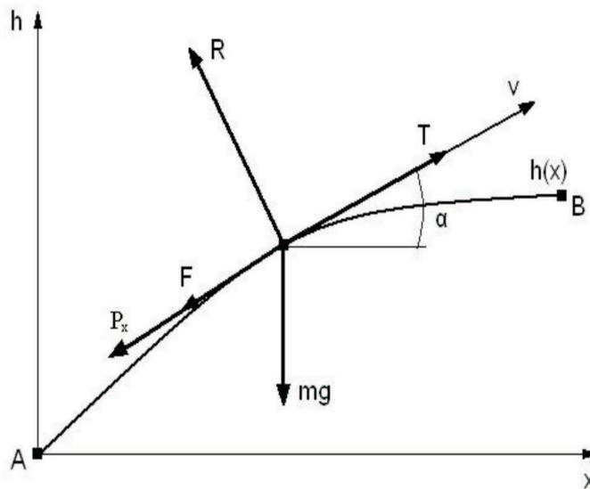
Fig. 1. Particle model of the vehicle
