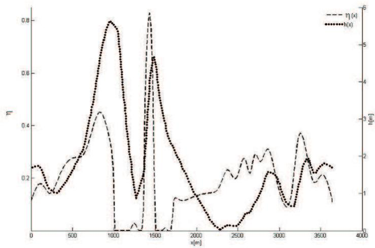
Fig. 5. Optimum throttle setting versus covered distance. The dotted line is the profile of the trace (cf. right-hand scale)
