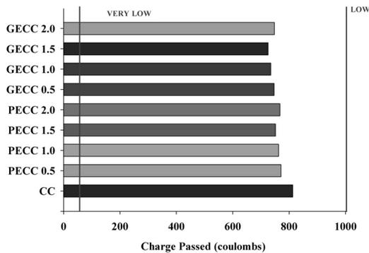
Fig 10. RCPT values of various mixes of ECC
