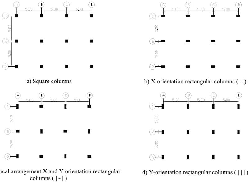
Fig. 2. Rectangular floor plan (ratio 1.5) models with different column arrangements and orientations
