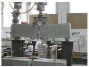
Fig. 4. Loss of bond of an HFRP bar in the final loading stage
