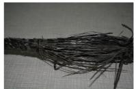
Fig. 2. 14 mm HFRP bars after rupture during a tensile test
