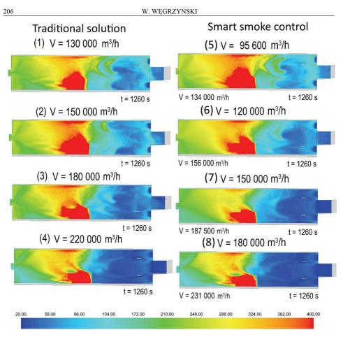
Fig.4. The temperature of smoke  $(20 - 400 \text{ }^{\circ}\text{C}$  and more) at the height of 2,00 m above the floor, for four traditional and four smart smoke control systems, as described in [7]. Systems on the right side did operate at approx. 30% lower operating pressure, than their traditional counterparts
