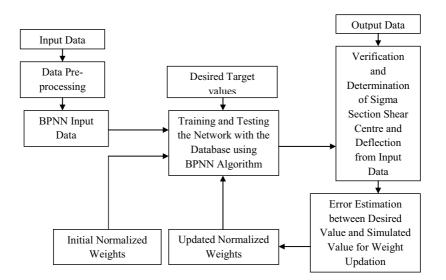
Fig. 3. Block Diagram of BPNN for the proposed model
