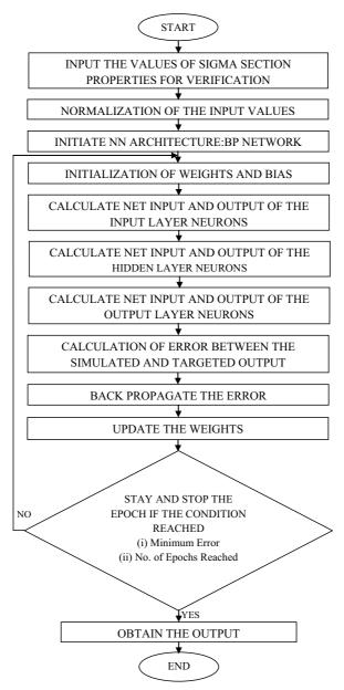
Fig. 2 Flowchart of BPNN Algorithm.
