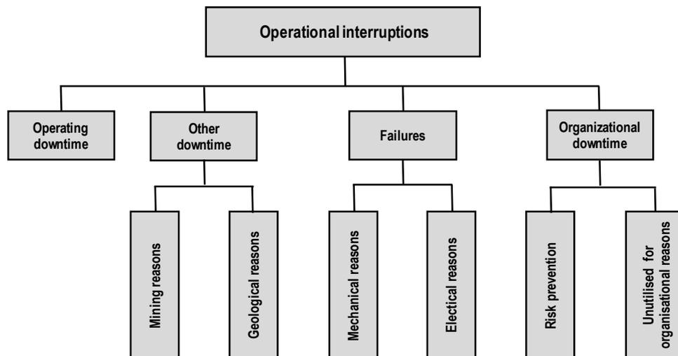
Fig. 2. Operating interruptions to mine face operations and their primary causes
