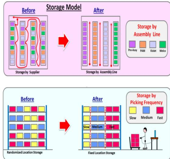
Fig. 3. The storage re-arrangement by assembly line and picking frequency.
