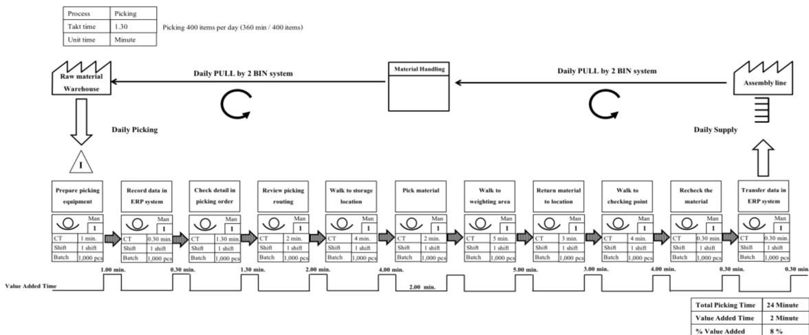
Fig. 1. Current state VSM of picking process.
