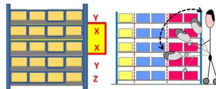
Fig. 4. The vertical storage re-allocation by picking frequency and ergonomics concept.
