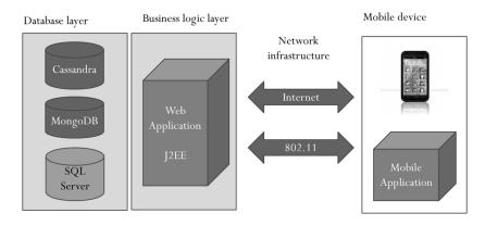
Fig 1. Three-layer architecture and access to databases.
