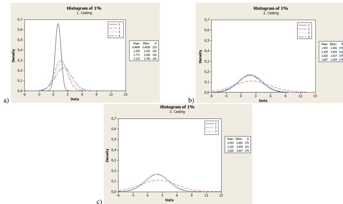
Fig. 6. Density distribution function of pores measured on the cross-section of reduced pressure test samples 1 wt% Ti added and recycled A356: a) 1<sup>st</sup> recycling, b) 2<sup>nd</sup> recycling, c) 3<sup>rd</sup> recycling
