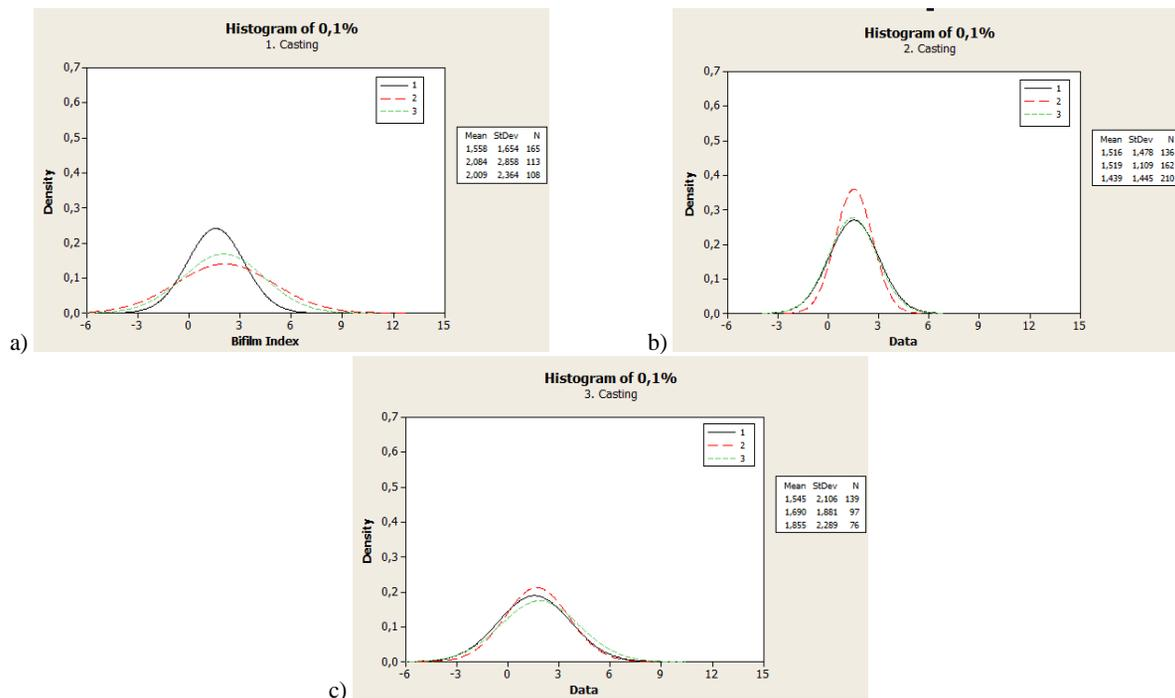
Fig. 5. Density distribution function of pores measured on the cross-section of reduced pressure test samples 0.1 wt% Ti added and recycled A356: a) 1<sup>st</sup> recycling, b) 2<sup>nd</sup> recycling, c) 3<sup>rd</sup> recycling
