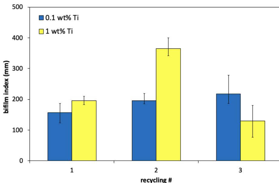
Fig. 2. Bifilm index of 3 times recycled 0.1 and 1 wt% Ti added A356
