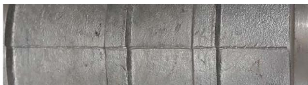
Fig. 4. Example of flash to be removed
