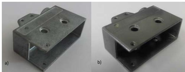
Fig. 1. View of surface faults on the tap casting used on the housing of micro switch [8]
