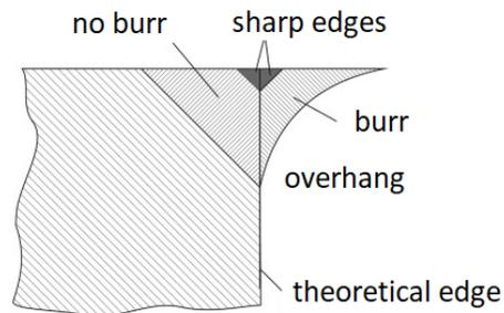
Fig. 2. Scheme of burr according ISO 13715 [22]
