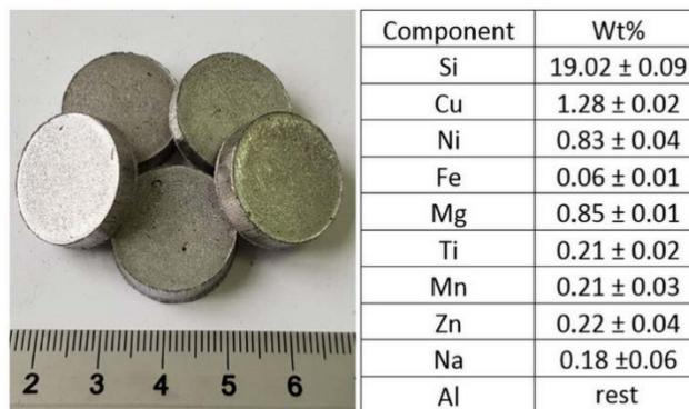
Fig. 2 The appearance of five compacts and its chemical composition
