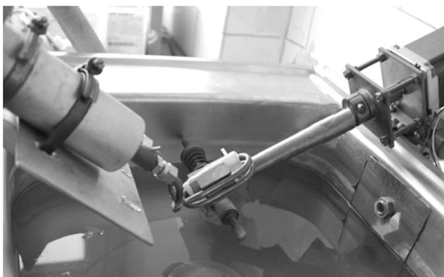
Fig. 2. The inductor (left) and the specimen holder (right)
