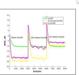
Fig. 6. Steady state MSE analysis of the proposed algorithm for echo cancellation application
