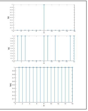
Fig. 4.Impulse response of sparse, semi sparse and non-sparse system
