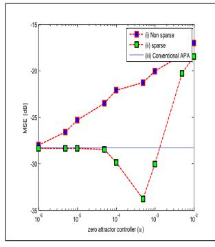
Fig. 2. Steady state MSE analysis of ZA-APA for sparse and non sparse system with different zero attractor controller
