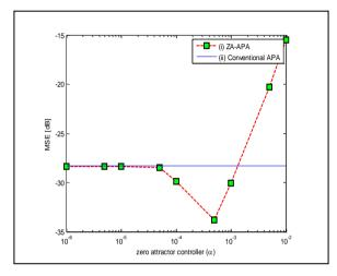
Fig. 1. Steady state MSE of ZA-APA with different zero attractor controller
