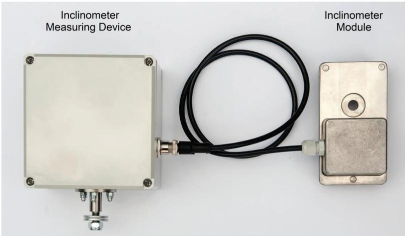
Fig. 3. Complete inclinometer device
