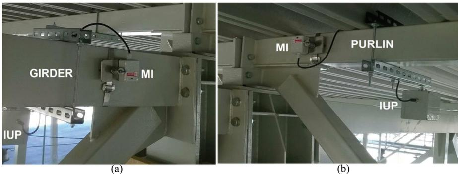
Fig. 4. Examples of inclinometer devices (IUP and MI) attachment to the girder (a) and truss purlin (b)
