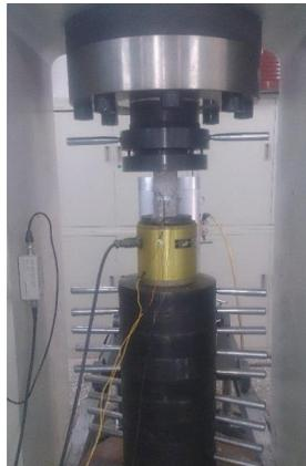
Figure 7. Rock sample placed in TAW-2000D Rock mechanics testing machine
