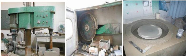
(a) Coring machine      (b) Cutting machine      (c) grinding machine
