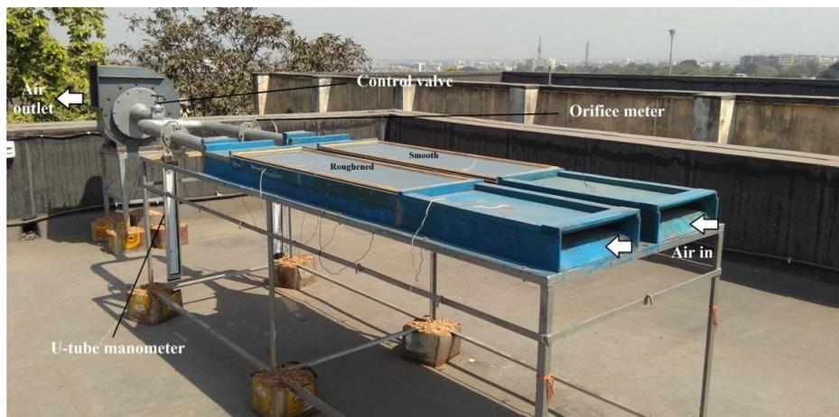
Figure 2: Pictorial view of SAH experimental setup.
