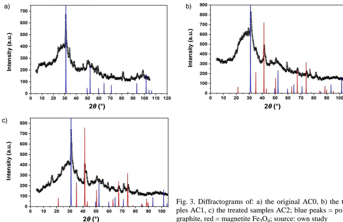
Fig. 3. Diffractograms of: a) the original AC0, b) the treated samples AC1, c) the treated samples AC2; blue peaks = polycrystalline graphite, red = magnetite Fe<sub>3</sub>O<sub>4</sub>; source: own study
