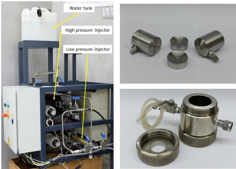
Fig. 2. Photograph of the water injection system including the pumping system and the Hoek cell and spherical seat bases with water distribution elements
