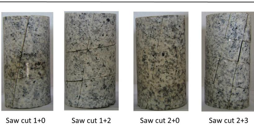
Fig. 5. Photograph of the different types of artificially fissured (saw-cut) joints
