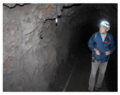
Fig. 1. Passive detector placed inside the gallery, where the workers spend their working hours
