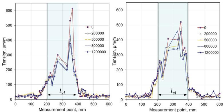
Fig. 9. Measured tension across the sleeper in pressure sensors sensors (left – standard grading, right – wide grading)
