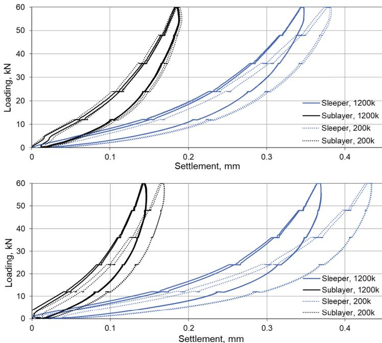
Fig. 12. Static stiffness of the whole ballast layer and the sublayer at the beginning and after 1,2 mio loading cycles (top – standard grading, bottom – wide grading)
