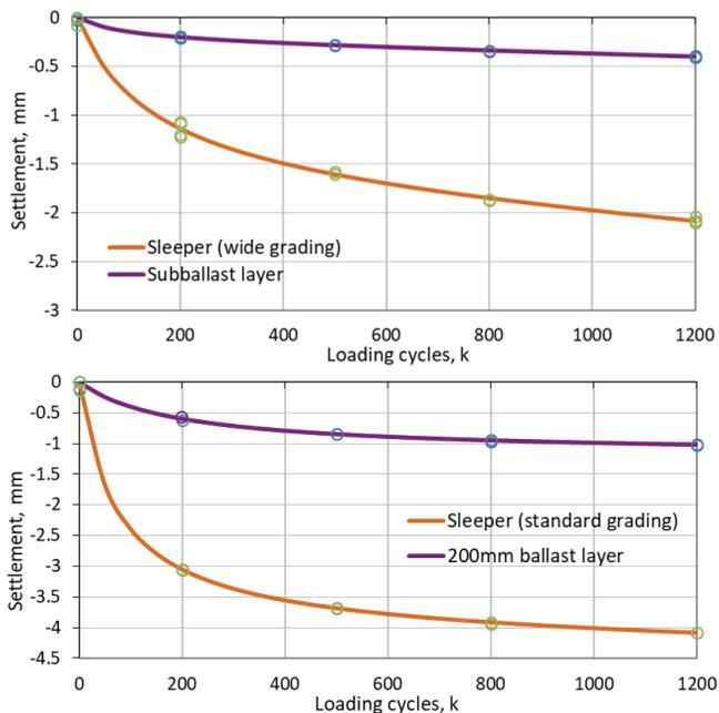
Fig. 5. The points of settlements measurements and the phenomenological model fitting for the reference ballast layer (top) and the double layer ballast
