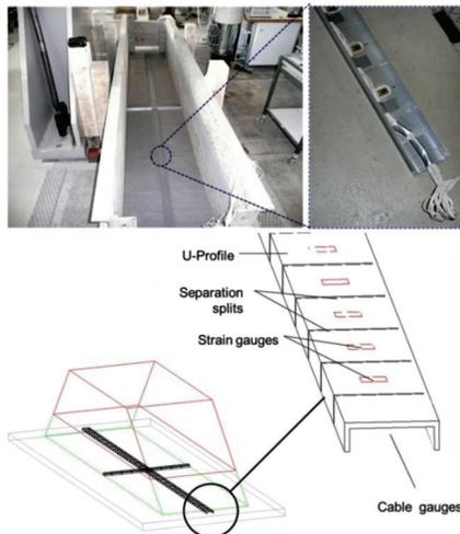
Fig. 2. Pressure measurement sensors setup and sensor location
