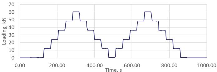
Fig. 11. Loading cycle for the ballast stiffness estimation test
