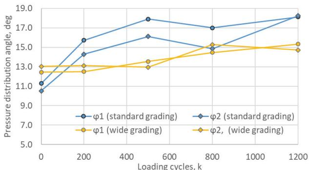
Fig. 10. Pressure distribution angles depending on the loading cycle
