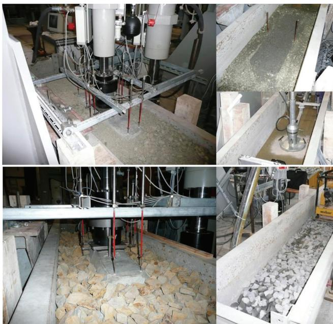
Fig. 3. Photographs of the laboratory tests (top: double layer ballast, bottom: standard ballast layer)
