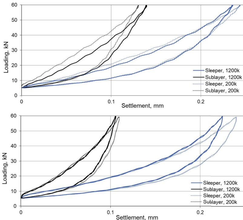
Fig. 13. Dynamic stiffness of the whole ballast layer and the sublayer at the beginning and after 1,2 mio loading cycles (top – standard grading, bottom – wide grading)
