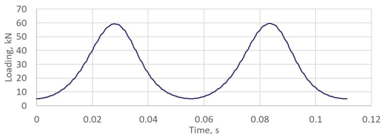
Fig. 4. Loading line of the sleeper for the 200-1200 thousand cycles
