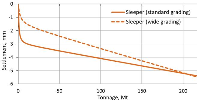
Fig. 7. Comparison of long-term settlement behaviour for upper layer of wide graded ballast and that of standard ballast
