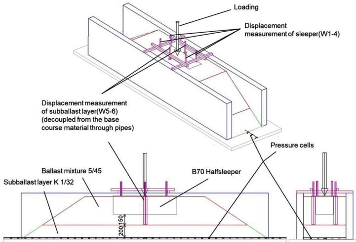
Fig. 1. Schematic view of the test set-up
