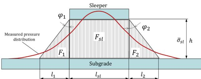
Fig. 8. The scheme for calculation of pressure distribution angle
