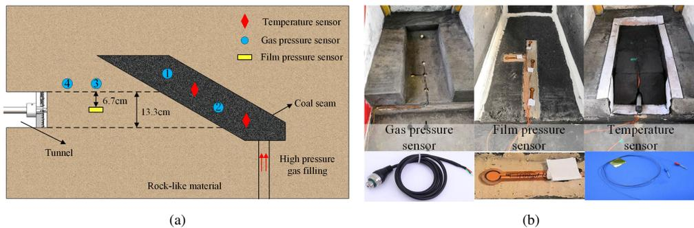
Fig. 9. Arrangement of some key sensors. a) Locations of selected key sensors. b) Sensor placing.
