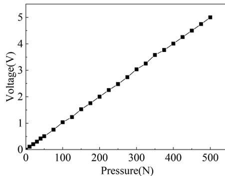
Fig. 3. Curve between the pressure and the output voltage.
