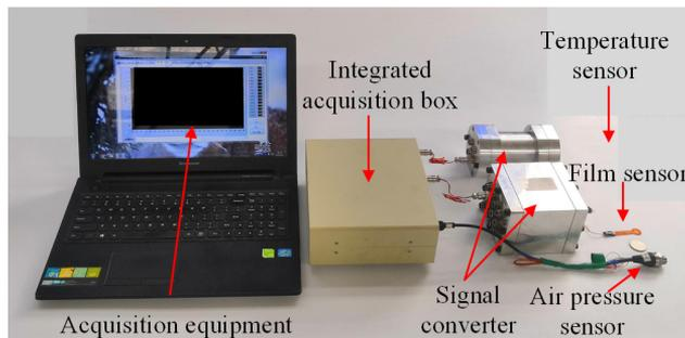
Fig. 5. Highly integrated acquisition module.
