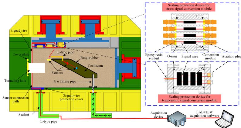
Fig. 6. The overall connection mode and principle.
