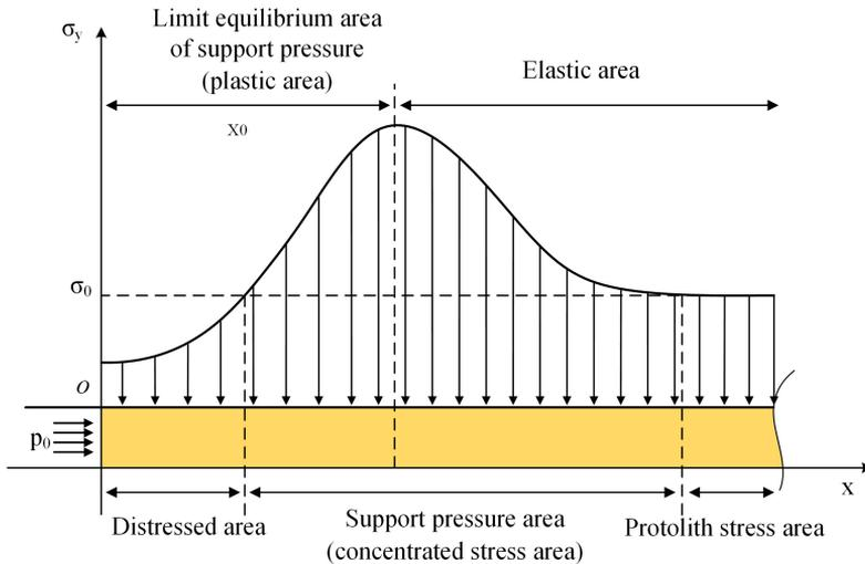
Fig. 13. Support pressure area in front of the tunneling face.
