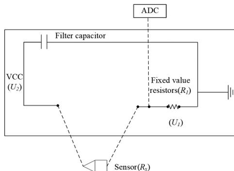
Fig. 2. Circuit design and the voltage sharing principle.
