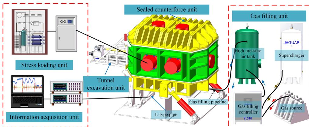
Fig. 8. Coal and gas outburst simulation test apparatus.
