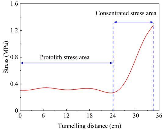
Fig. 12. Geostress curve in front of the tunneling face.
