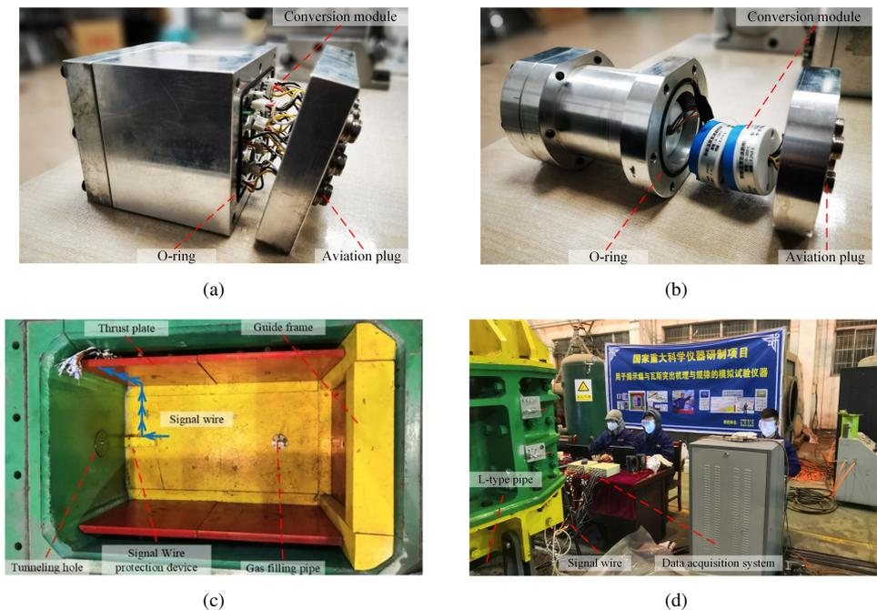
Fig. 7. Details of the hyperbaric resistant sealing protection technology. a) Sealing device for signal conversion module of film sensor. b) Sealing device for signal conversion module of temperature sensor. c) Signal wire arrangement inside the apparatus. d) Signal wire arrangement outside the apparatus.
