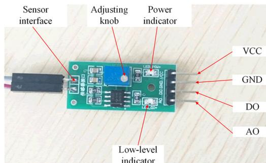
Fig. 4. Signal conversion module.
