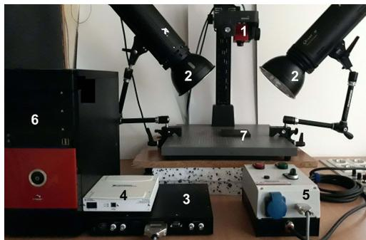
Fig. 2. Experimental setup for stepped heating method.
