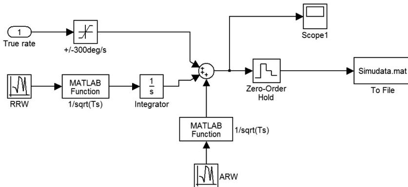
Fig. 4. The Simulink model for generating outputs of the gyroscope array signals.
