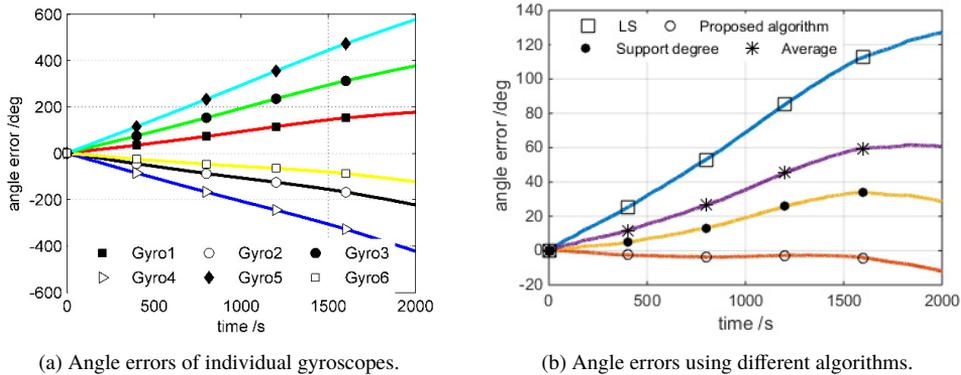
Fig. 6. Integration angle error before and after fusion.
