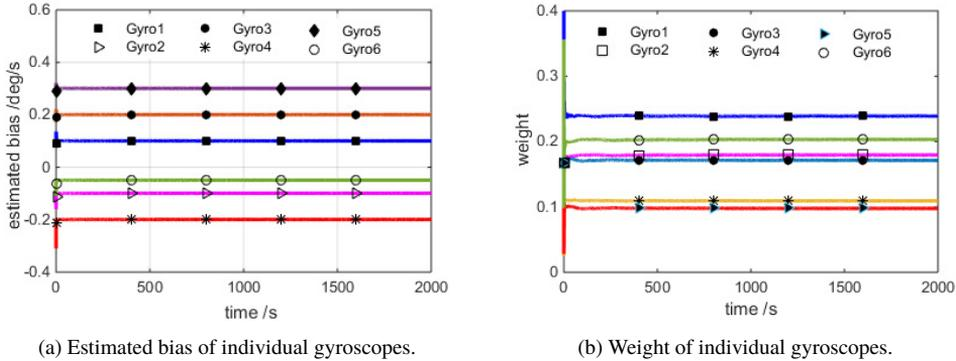
Fig. 7. Parameter estimation of the gyroscope arrays in the static simulation.
