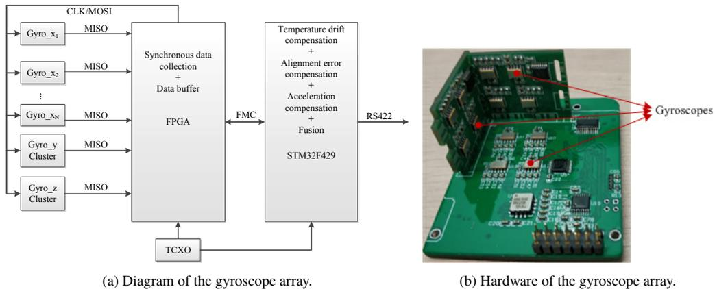
Fig. 2. An implementation of the gyroscope array.
