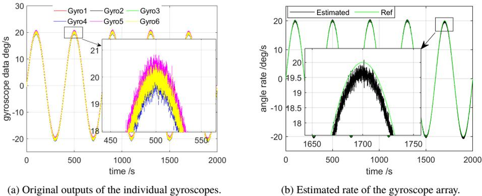
Fig. 8. Sinusoidal rate simulation of the gyroscope array.
