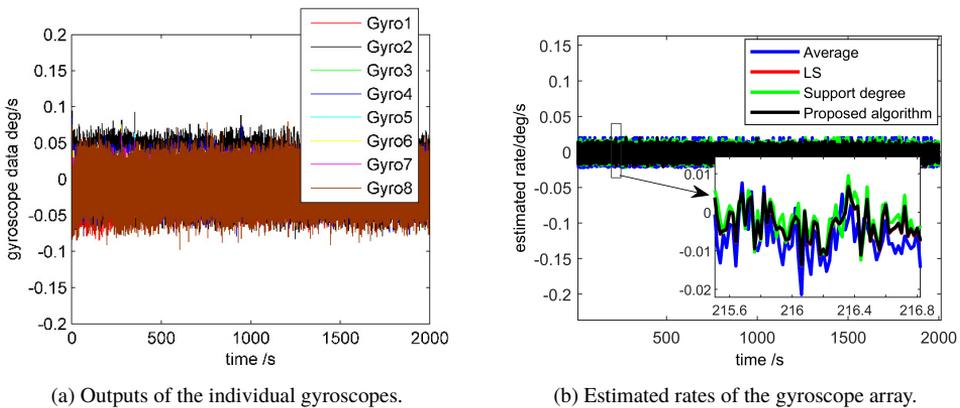
Fig. 12. Results of the static test.
