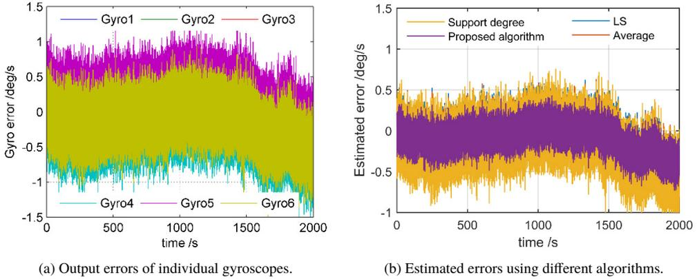
Fig. 9. Error comparison before and after fusion.
