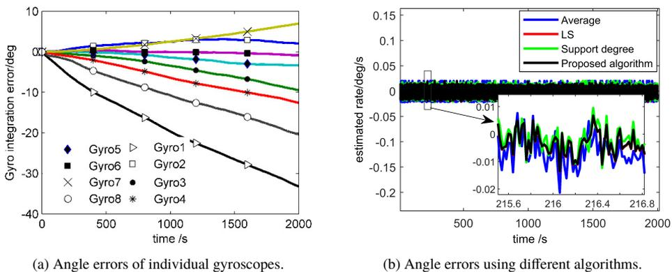
Fig. 13. Integration angle error before and after fusion.
