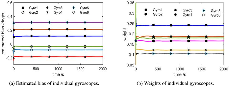
Fig. 10. Parameter estimation of the gyroscope array in the dynamic simulation.
