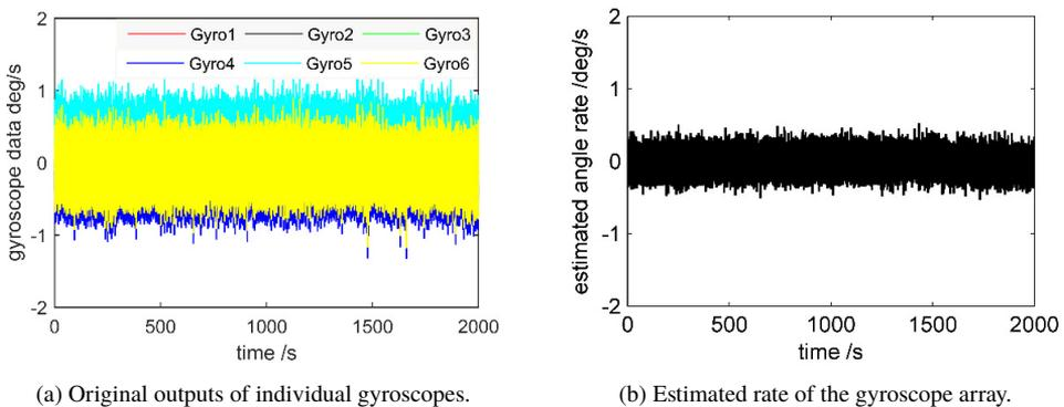
Fig. 5. Static simulation of the gyroscope array.
