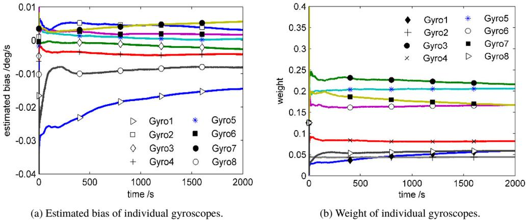
Fig. 14. Parameter estimation of the gyroscope arrays in the static experiment.
