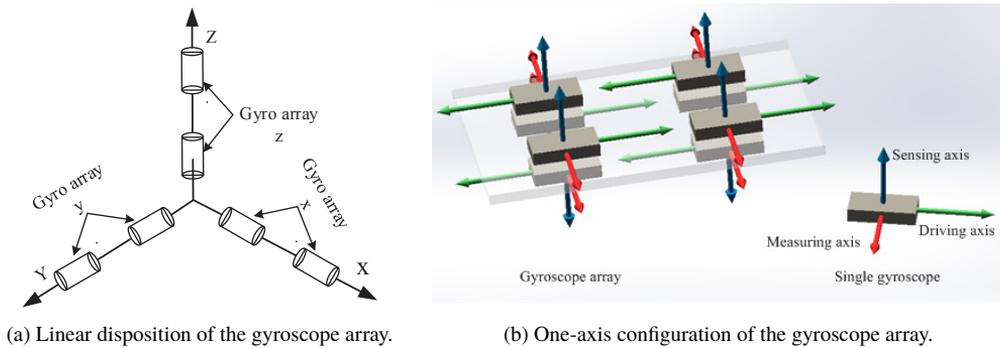
Fig. 1. Configuration of the gyroscope array.
