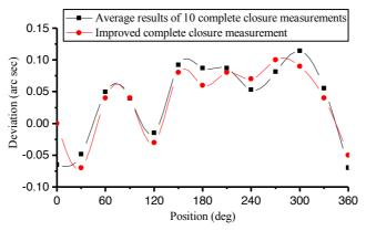
Fig. 3. The position error of the angle comparator.
