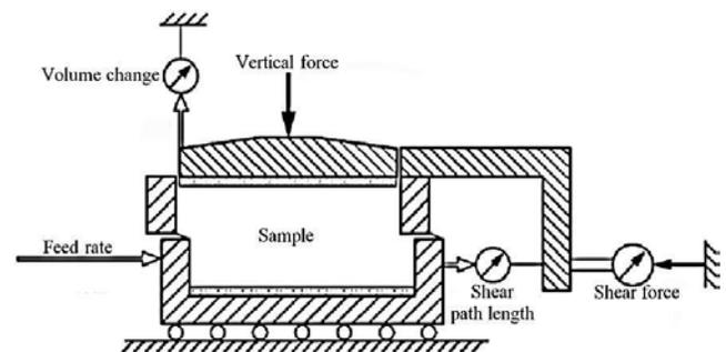
Fig 2: Principle of direct shear test [12]
