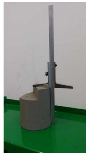
Fig 11: Displacement measurement of sand sample
