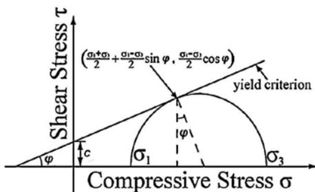
Fig 1: Mohr–Coulomb's fracture criterion [11]
