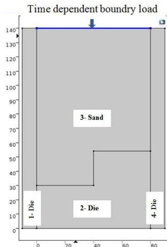
Fig 5: Geometry of the sand sample and die
