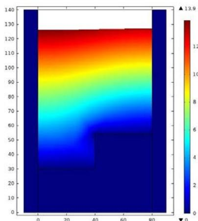
Fig 10b: Displacement of sand sample @ 0.5sec
