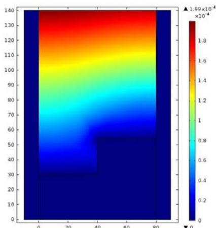
Fig 10a: Displacement of sand sample @ 0.01sec
