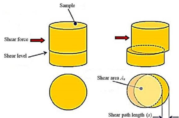
Fig 3: Shear area during shearing process [12]
