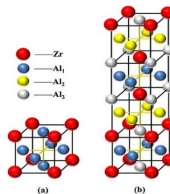
Fig. 2. Forms of the  $Al_3Zr$  intermetallic phase precipitation in the crystallographic lattice: a)  $L1_2$  b)  $DO_{23}$  [10]
