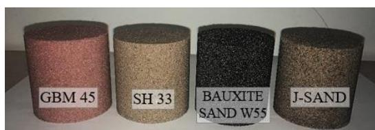
Fig. 4. Standard permeability test specimens
