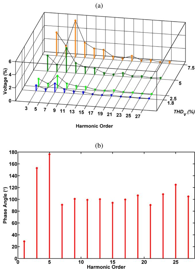
Fig. 2. Harmonics spectra of the supply voltage used during the measurements and their phase angle
