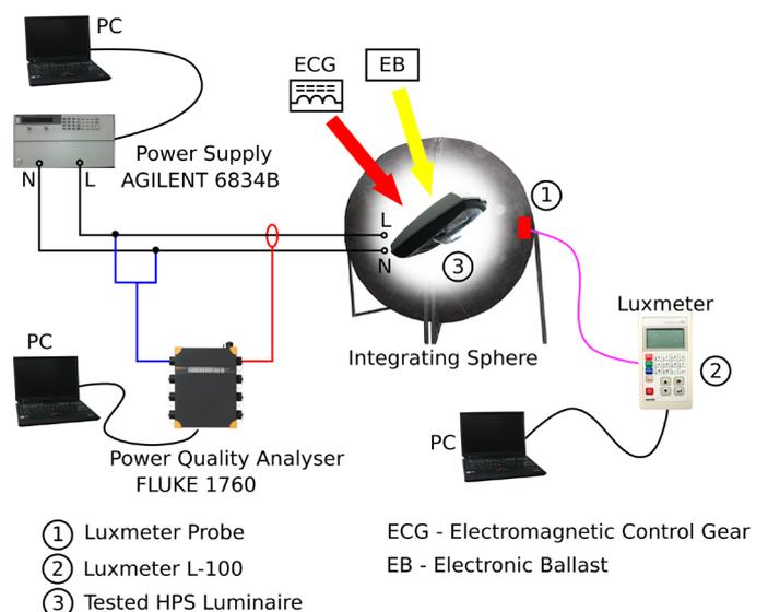
Fig. 1. Experimental setup for HPS luminaire with electromagnetic control gear and electronic ballast
