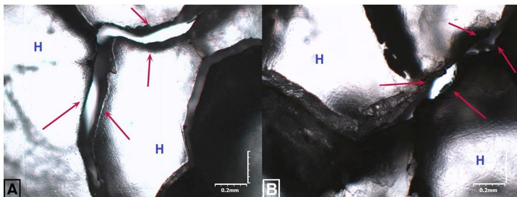
Fig. 3. The cracks at the crystal boundaries in a pink rock salt samples (double polished sections about 1-3 mm thick, parallel nicols) from the Kłodawa salt dome after uniaxial compression tests:
