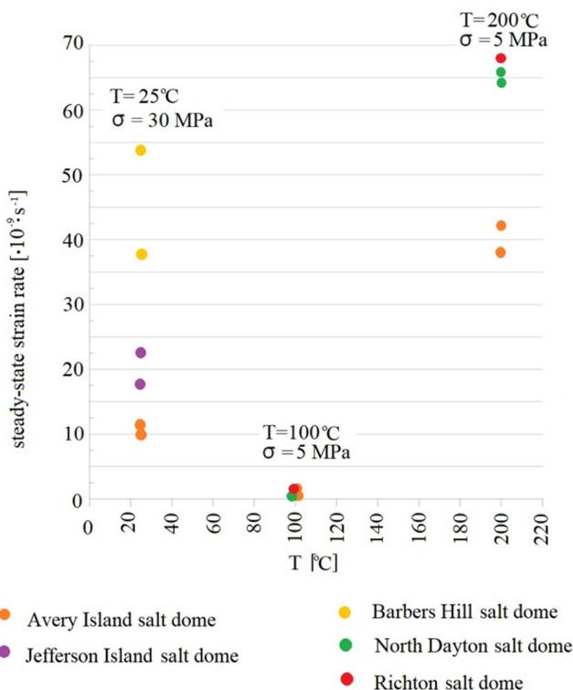
Fig. 11. The steady state creep rates for rock salt from different salt domes in USA [110]
