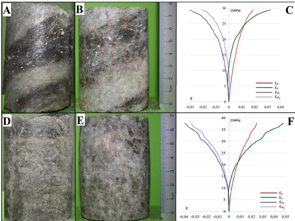
Fig. 8. Rock salt samples characterised by unevenly distributed impurities from the Łęzkowice salt deposit ([63] modified): A-C banded rock salt, D-F – grey salt with unevenly distributed impurities within halite grains, A, D before tests, B, E – after uniaxial compression test, C, F, stress-strain characteristics
