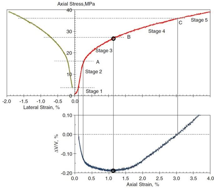
Fig. 1. The general stress-strain relationship for a rock salt sample from the Asse salt dome [50]
