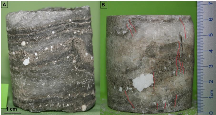
Fig. 4. The rock salt sample with claystone interlayers from the Łęzkowice salt deposit:
