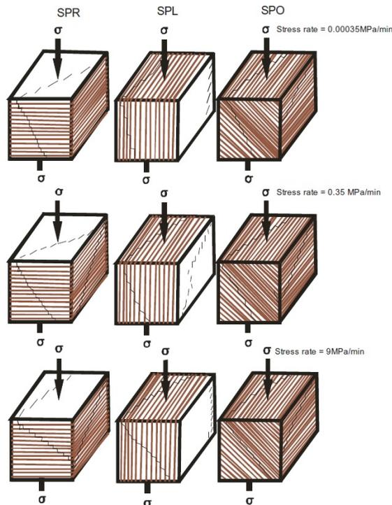
Fig. 5. Crack patterns developed in samples deformed perpendicular, parallel, and oblique to bedding [43]
