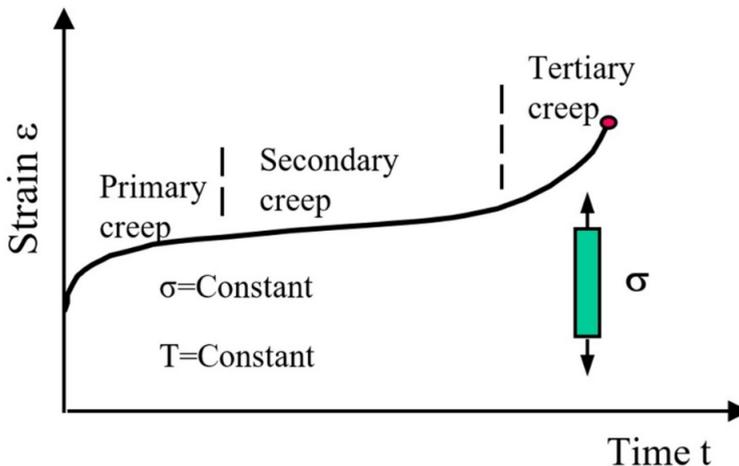
Fig. 10. Idealized creep curve showing three creep stages [96]
