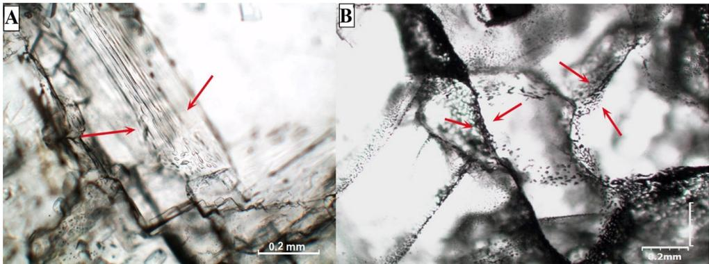
Fig. 9. Fluid inclusion plains at halite grain boundaries: A – rock salt from LGOM (double polished sections about 1–3 mm thick, parallel nicols) rock salt, B – pink rock salt from the Kłodawa salt dome
