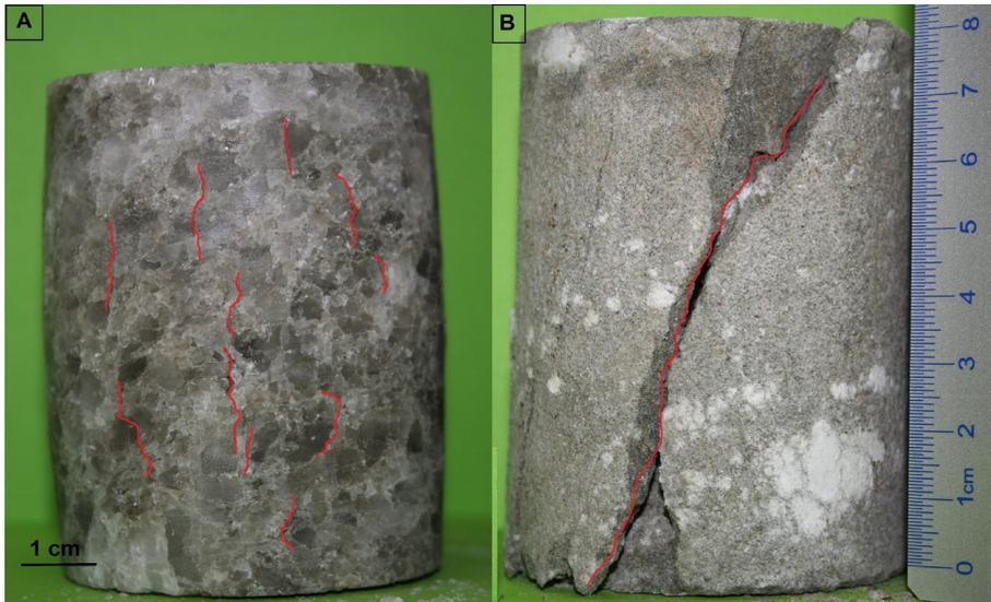
Fig. 6. Comparison between failure mode of rock salt and salty claystone from the Łężkowice salt deposit:
