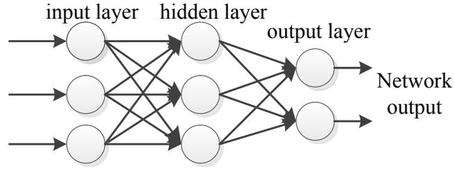
Fig. 3. Topological structure of wavelet neural network
