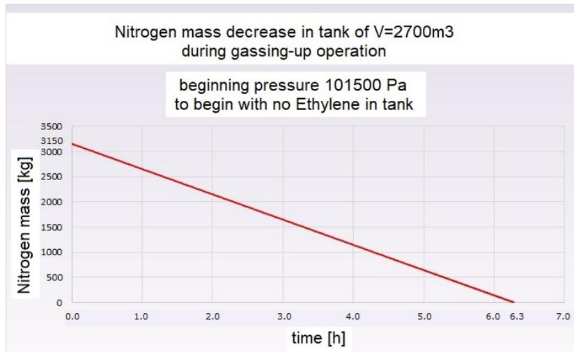
Figure 2: Decrease of nitrogen amount in tank as a function of gassing-up operation time.
