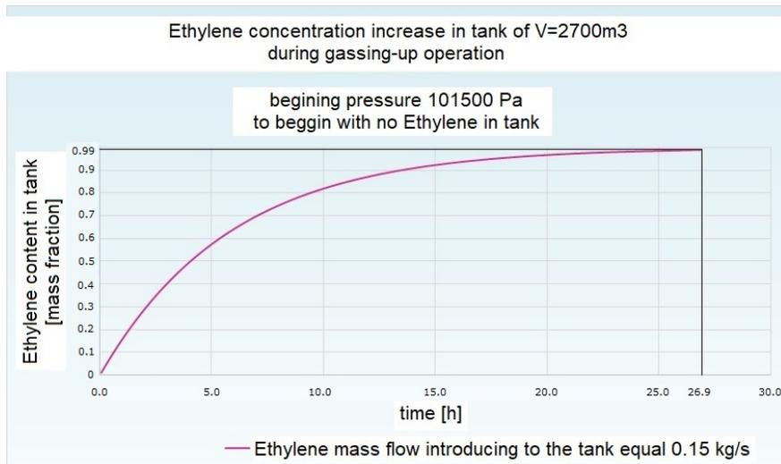
Figure 4: Increasing the amount of ethylene in the tank as a function of gassing-up time (without increasing the tank pressure by introducing the ethylene vapour).
