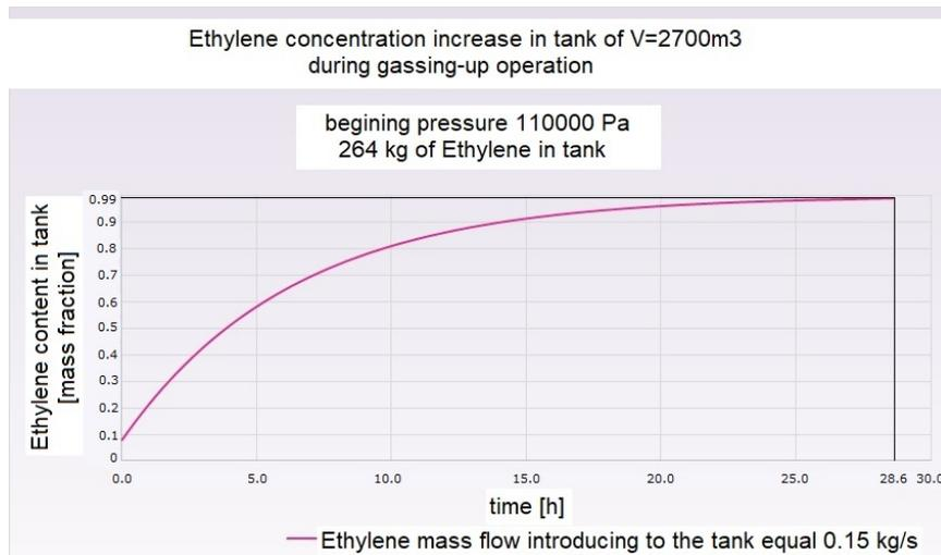
Figure 9: Ethylene amount increase in tank as a function of time (after introducing 264 kg of ethylene to increase the tank pressure).
