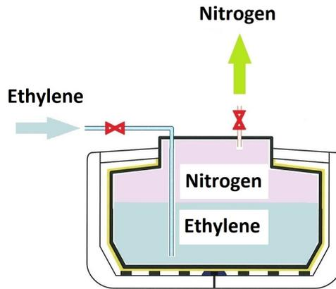
Figure 1: Nitrogen ‘pushing out’.
