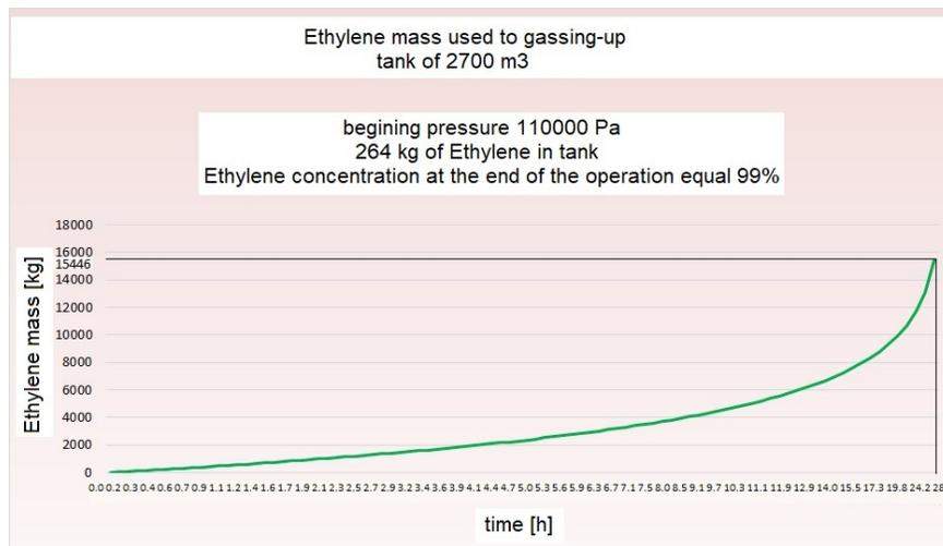
Figure 10: The amount of ethylene used to carry out the gassing-up process as a function of time (after introducing 264 kg of ethylene to increase the tank pressure).
