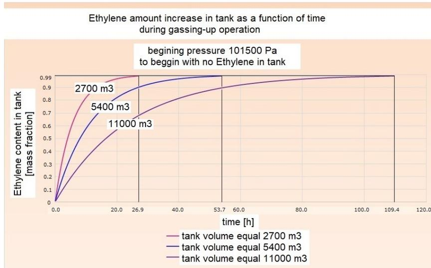
Figure 6: The increase of the amount of ethylene in the tank as a function of time of gassing-up for different values of the tank volume,  $V_z$ , without increasing the tank pressure by introducing the ethylene vapour.
