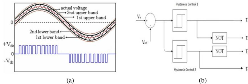
Fig. 2. Principle of hysteresis controller (a); switching signals (b)
