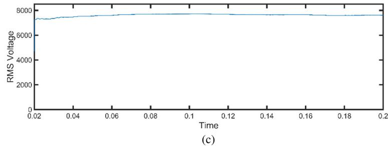
Fig. 9. RMS voltage in the presence of IPFC, when the load is increased suddenly at 0.1 seconds; (a), (b) and (c) with IPFC-hysteresis for R, Y, B phases, respectively
