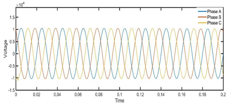
Fig. 8. Voltage of line 1, when the load is increased suddenly at 0.1 seconds in the presence of IPFC-PR
