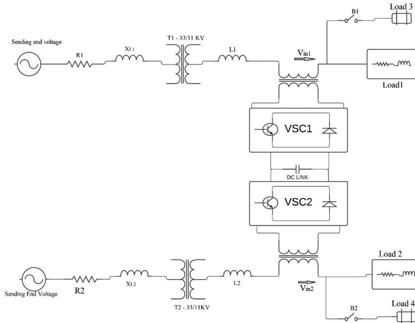
Fig. 4. Basic line diagram of IPFC
