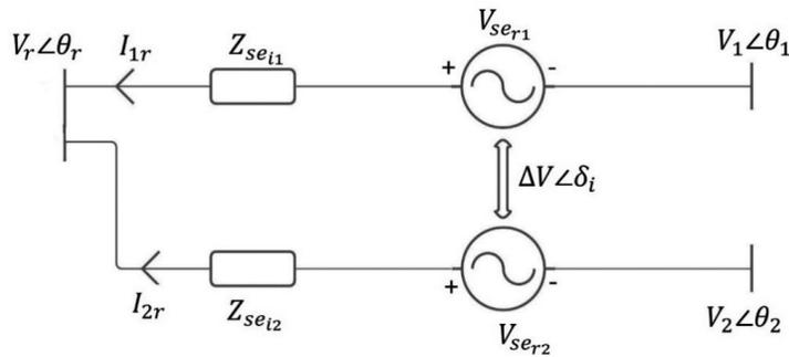
Fig. 1. IPFC power injection model
