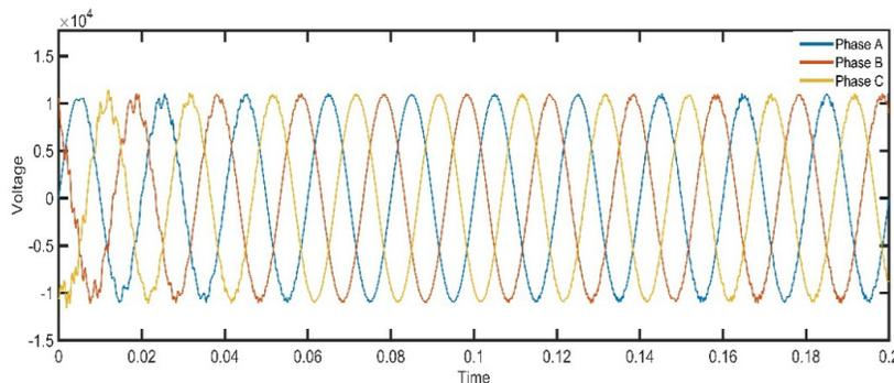
Fig. 7. Voltage of line 1 when the load is increased suddenly at 0.1 seconds in the presence of IPFC-hysteresis
