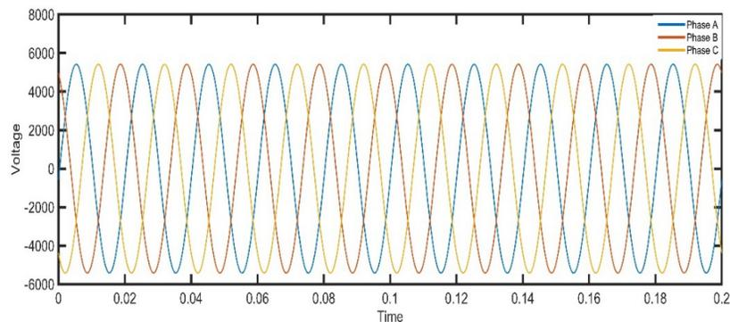
Fig. 5. When IPFC is not connected, voltage at the end of transmission line 1
