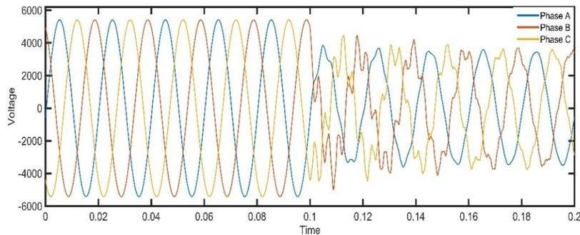
Fig. 6. Voltage at the end of transmission line 1, when the load is increased suddenly at 0.1 seconds in the absence of IPFC
