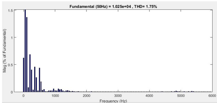
Fig. 11. THD of the system with IPFC-PR
