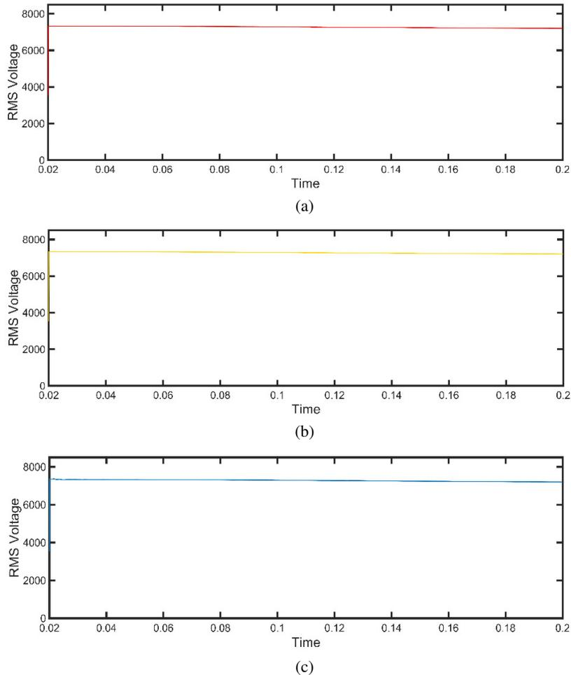
Fig. 10. RMS voltage in the presence of IPFC, when the load is increased suddenly at 0.1 seconds; (a), (b) and (c) with IPFC-PR for R, Y, B phases, respectively
