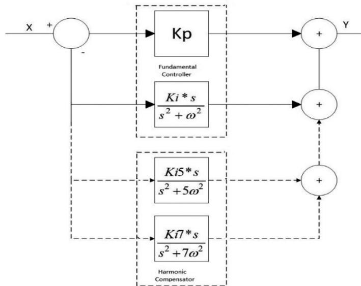
Fig. 3. PR controller and harmonic compensator structure
